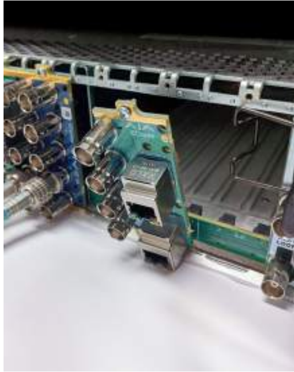
Figure 6. Rear Card Inserting Into Frame Seating Slot
