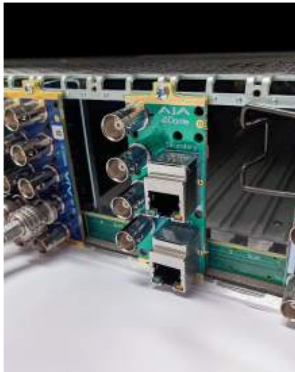
Figure 7. Rear Card Inserted Into Frame Seating Slot
