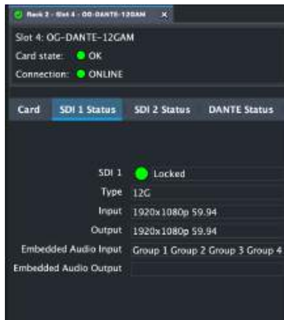
Figure 5. Signal is present and locked
