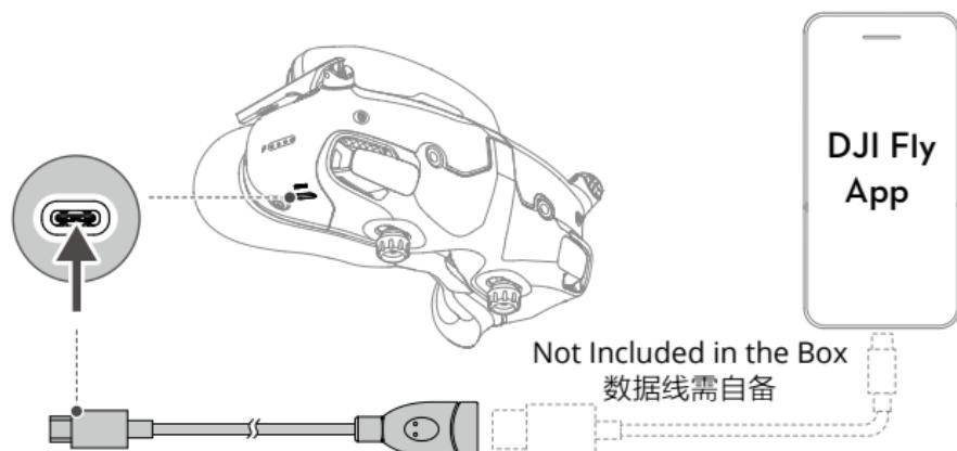
**EN** Connect the USB-C port of the goggles to the mobile device with the USB-C OTG cable and a suitable data cable. Run DJI Fly on the mobile device and follow the prompts to activate the DJI devices.
