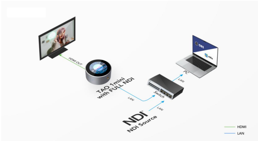
NDI Decoding Connection Diagram
