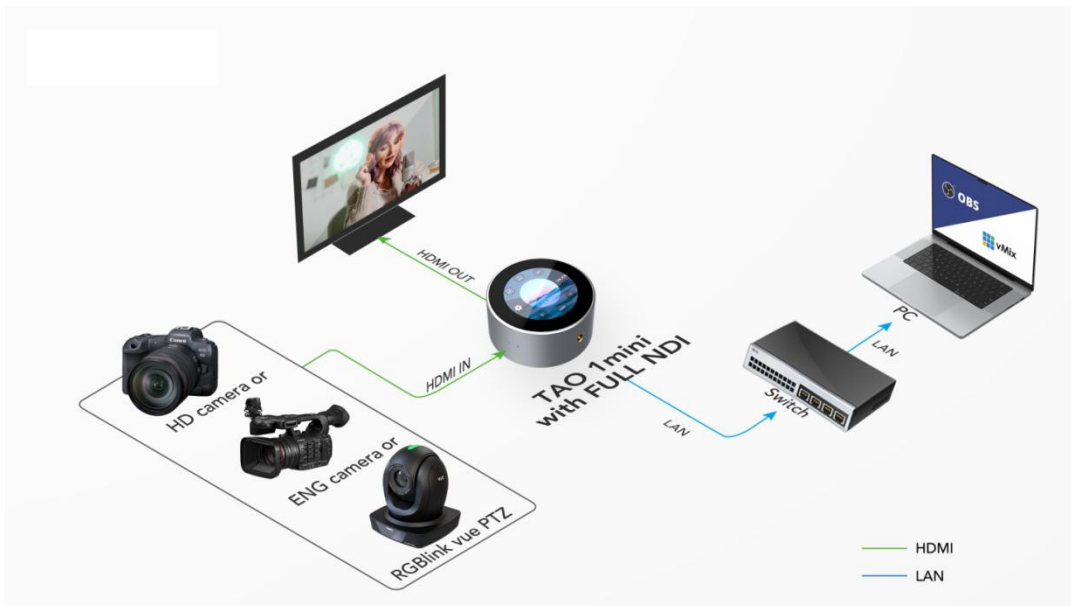
NDI Encoding Connection Diagram
