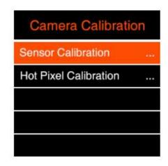
3. Select the one you want and press **OK** button to start it. PLEASE WAIT until the calibration processing is finished and **DO NOT INTERRUPT IT!**
