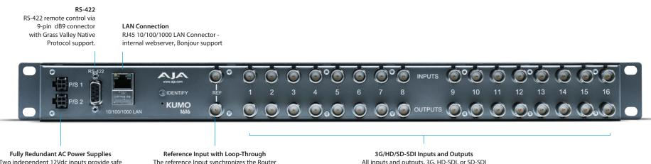
Two independent 12Vdc inputs provide safe operations. Power status can be checked from a LAN attached browser.
