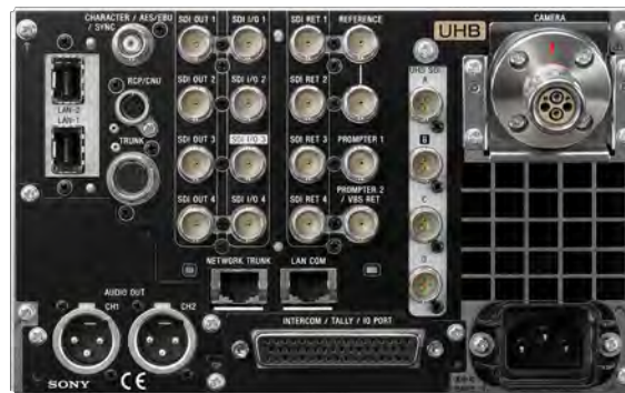
HDCU-5500 Rear view ST 2110 IP interface with optional HKCU-SFP50
