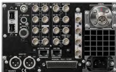
HDCU-3500 Rear view ST 2110 IP interface with optional HKCU-SFP50
